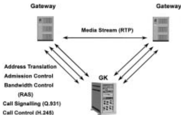
Fig. 10. Gatekeeper routed call signaling (Q.931/H.245).
