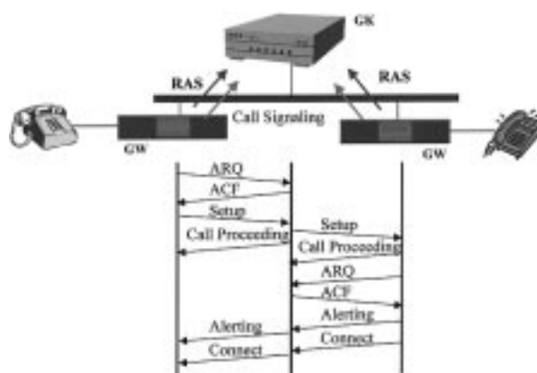
Fig. 12. Basic call setup with gatekeeper routed call signaling.
