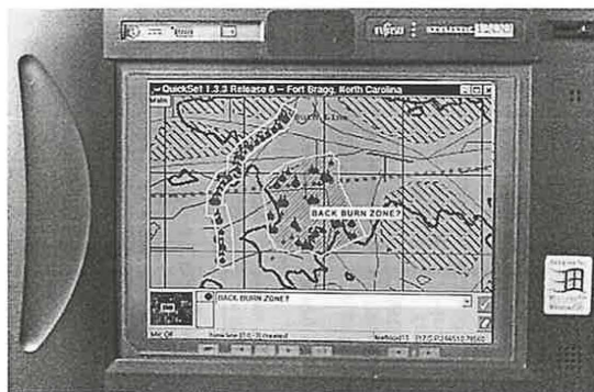
Figure 5. QuickSet system running on a wireless handheld PC, showing user-created entities on the map interface.
