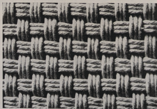
FIG. 90 Plain weave with tripled warps and wefts (sometimes called '3/3 basket' or '3/3 matt' weave).
