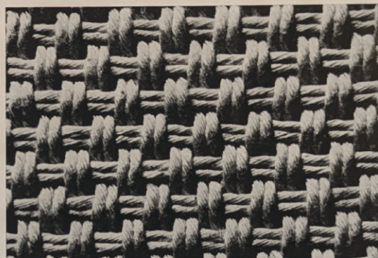
FIG. 89 Plain weave with paired warps and wefts (sometimes called 'basket' or 'matt' weave).
