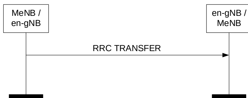
Figure 8.7.12.2-1: RRC Transfer procedure, successful operation.
