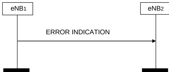
Figure 8.3.2.2-1: Error Indication, successful operation.
