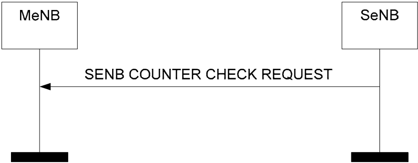
Figure 8.6.7.2-1: SeNB Counter Check procedure, successful operation.
