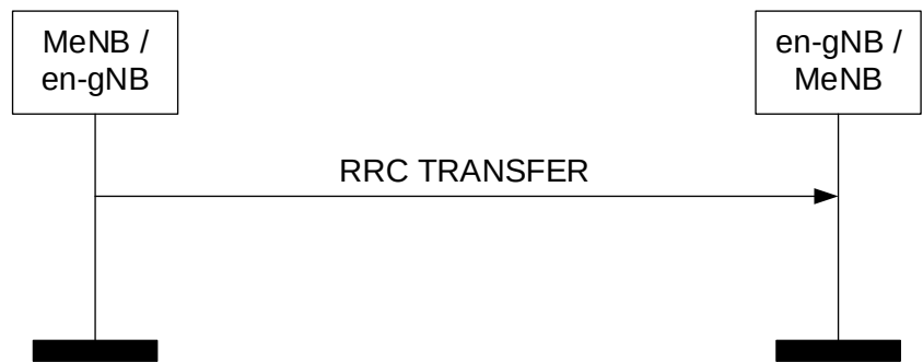
Figure 8.7.12.2-1: RRC Transfer procedure, successful operation.
