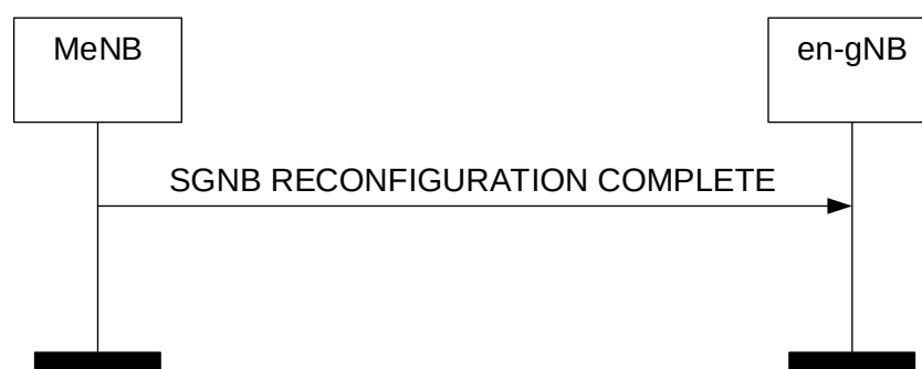
Figure 8.7.5.2-1: SgNB Reconfiguration Complete procedure, successful operation.
