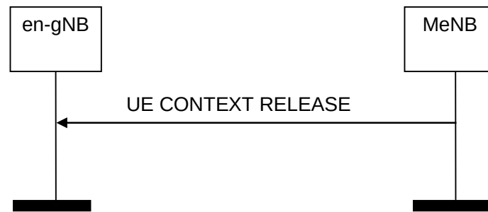
Figure 8.2.3.2-3: UE Context Release, successful operation for EN-DC
