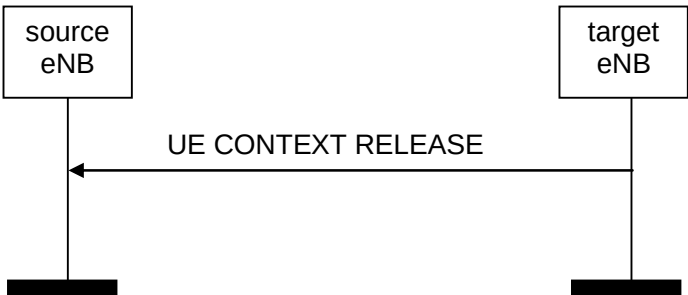
Figure 8.2.3.2-1: UE Context Release, successful operation for handover
