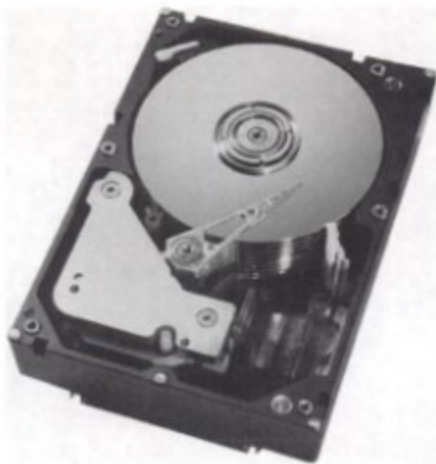
Figure 1-1 - An internal view of a standard SCSI drive.
