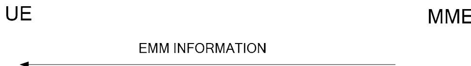
Figure 5.4.5.2.1: EMM information procedure
