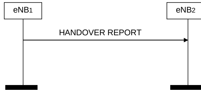
Figure 8.3.10.2-1: Handover Report, successful operation
