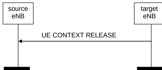
Figure 8.2.3.2-1: UE Context Release, successful operation for handover
