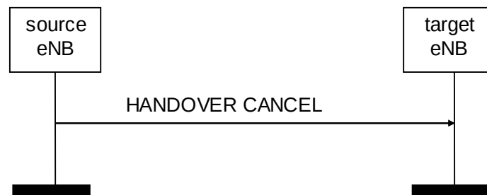
Figure 8.2.4.2-1: Handover Cancel, successful operation
