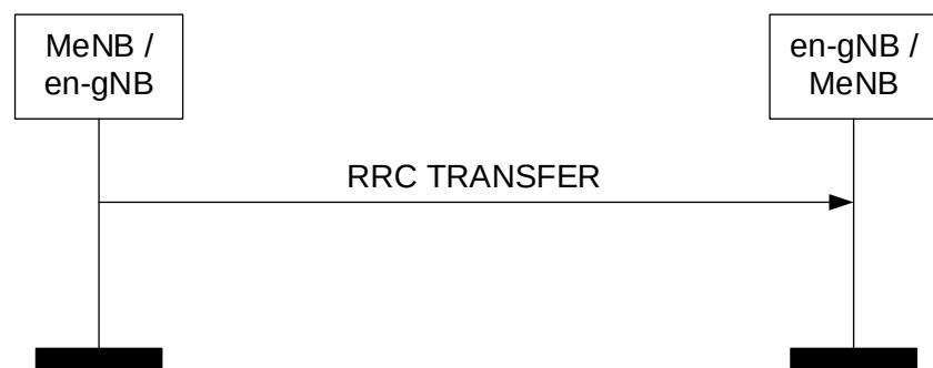
Figure 8.7.12.2-1: RRC Transfer procedure, successful operation.
