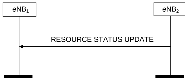
Figure 8.3.7.2-1: Resource Status Reporting, successful operation
