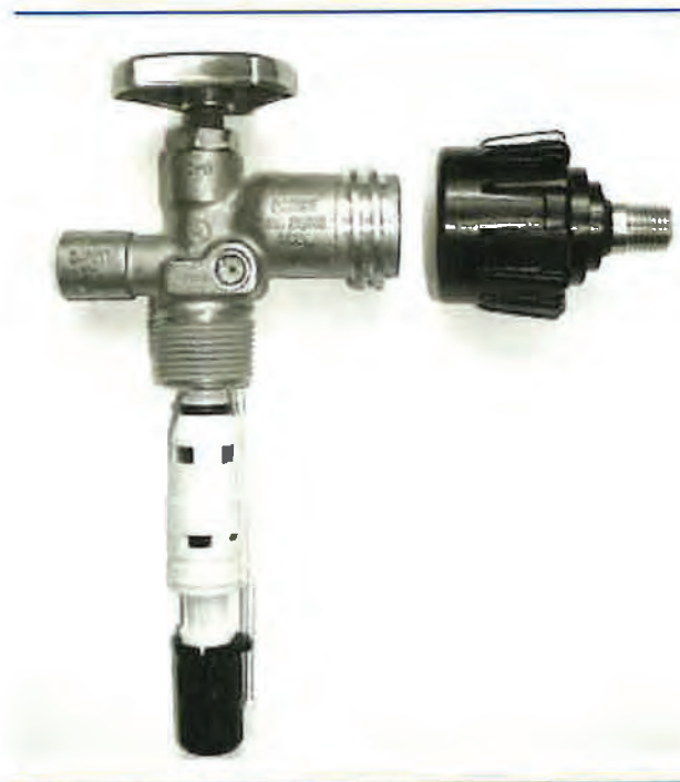
EXHIBIT 5.29 Cylinder Valve with Overfilling Prevention Device. Note the triangle-shaped hand wheel, which identifies the OPD valve. In addition to the unique hand wheel, the valve is also stamped "OPD." (Courtesy of Sherwood, Harsco Gas & Fluid Control Group)
