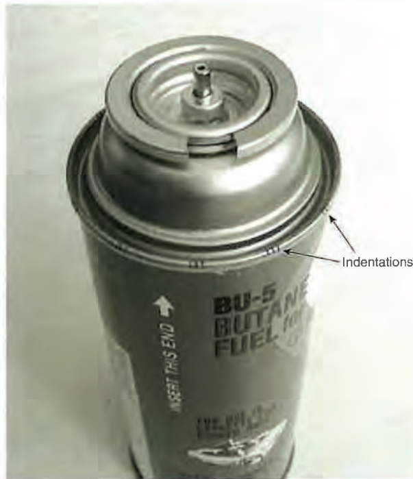
EXHIBIT 5.20 Indentations on the Upper Rim Seal of a Listed Butane Cylinder.
