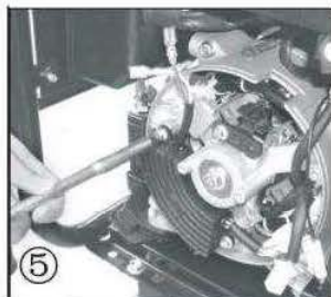
⑤ Install the new AVR with the 2 bolts (M5x16).
