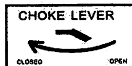
Figure 7 - Choke in the close position
