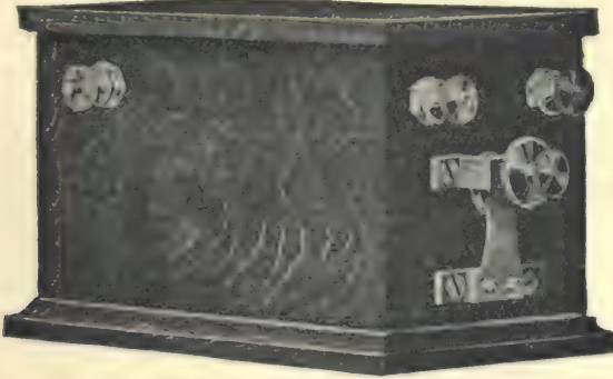
FIG. 13-12. — Three-Terminal Spark Coil.
