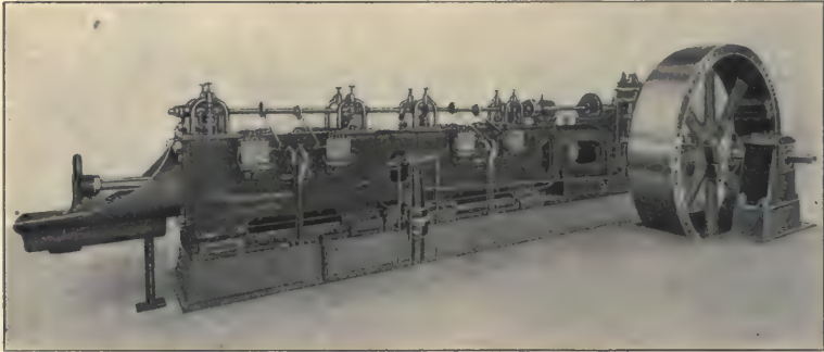
FIG. 12-63. — Riverside Heavy Duty Double-acting Tandem Gas Engine.
