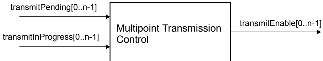
Figure 64-5—Multipoint Transmission Control Service Interfaces
