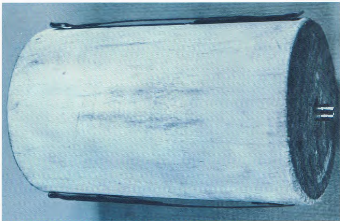
Fig. 19—A wooden arbor with two 1/4-inch metal strips fits snugly inside the paper tube core of each Blue "C" spandex package.
