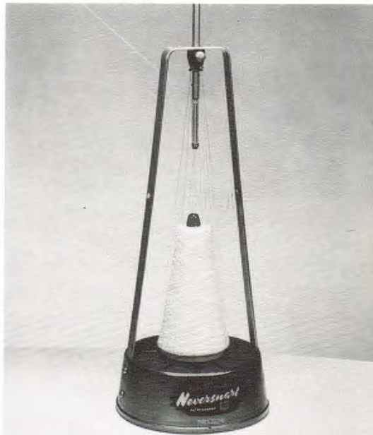
Fig. 24—The Mellor Bromley Neversnarl —just one of the several devices used for tensioning yarn spun with a core of Blue "C" spandex on the side of the cone.
