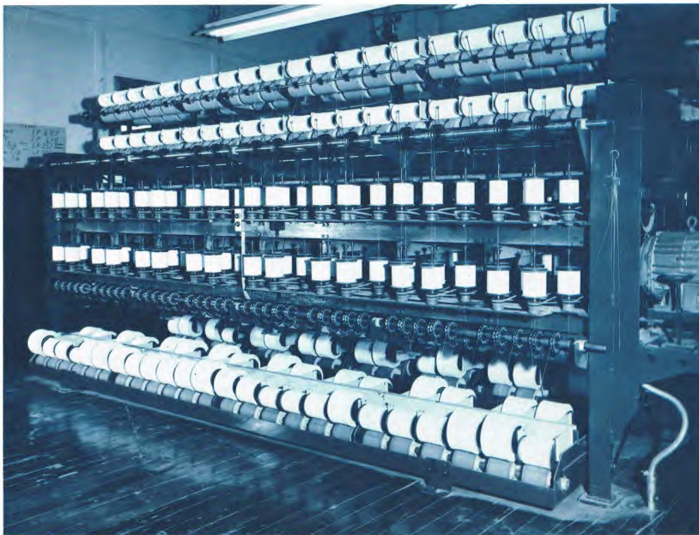
Fig. 9—The Arnold Conventional Flyer Type Covering Machine, a machine used extensively in the U.S. for the covering of Blue "C" and other spandex yarns.
