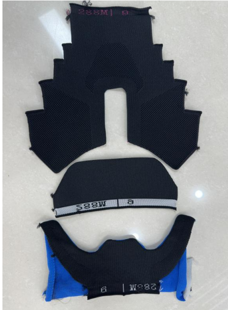
▲ Fabric count and structure of the upper when taken apart
