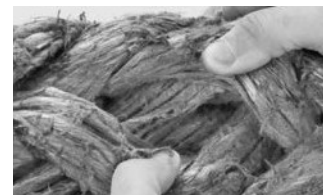
Inspect for internal abrasion
