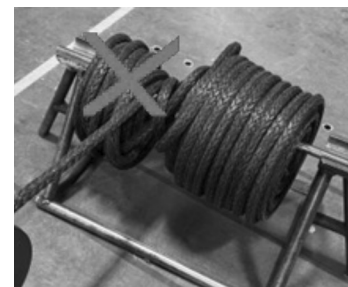
Do NOT unload a coil by placing a pipe through the bore, this will cause the coil to collapse.
