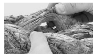
Inspect for pulled strands
