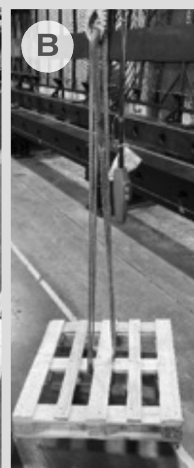
Coil and pallet (A) lifted slightly off the deck, allowing for free rotation during uncoiling. (B) Rope routing through pallet around structural elements.
