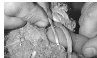
Compare surface yarns with internal yarns
