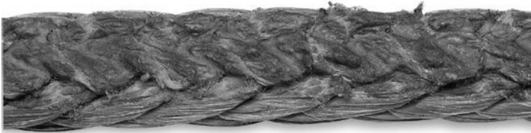
Melting damage on AmSteel®Blue
