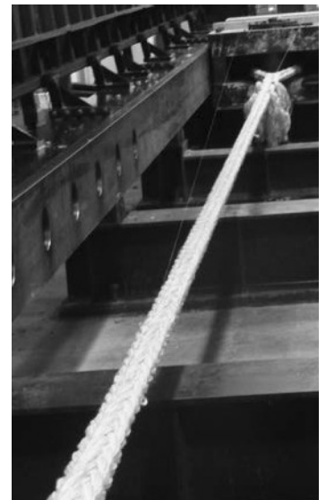
Samson's computer-controlled rope test bed records precise elongation measurements.
