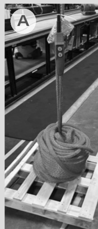
Coil and pallet (A) lifted slightly off the deck, allowing for free rotation during uncoiling. (B) Rope routing through pallet around structural elements.
