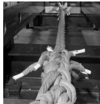
1.1 million pound tensile test machine
