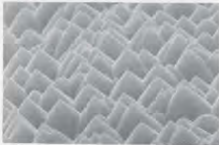
Figure 7.6. Appearance of a textured silicon surface under a scanning electron microscope. The peaks are typically 10\ \mu\text{m} high and are the tops of square-based pyramids. The sides of these pyramids are intersecting (111) planes within the crystal structure of the silicon.
