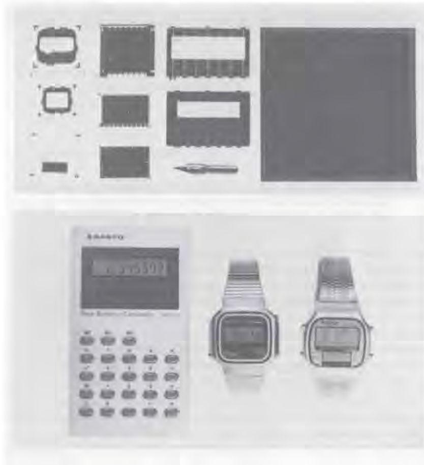
Figure 10.4. (a) First commercial amorphous silicon solar cell arrays designed for use in consumer products. (b) Calculator and watches powered by these arrays. (Photographs courtesy of Sanyo Electric Co. Ltd.)
