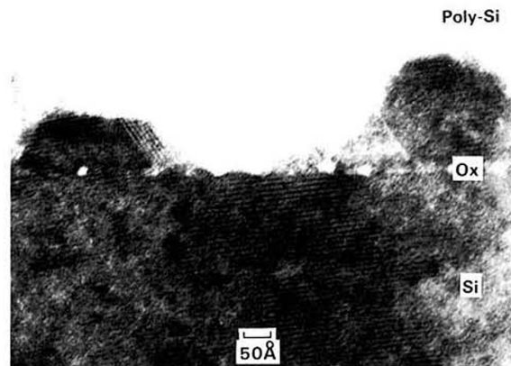
Fig. 4 HF specimen after 5 \times 10^{15} \text{cm}^{-2} As^+ , 900^\circ\text{C} 15min Note complete oxide break-up and extensive epitaxial re-alignment
