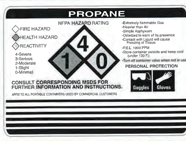
EXHIBIT 5.17 Sample Warning Label Intended for Use on Cylinders in Commercial or Industrial Service. (Courtesy of Screen Graphics of Florida)
