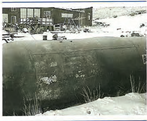
EXHIBIT 5.7 ASME Container Damaged by Fire. (Courtesy of Independent Propane Co., Pine, CO)
