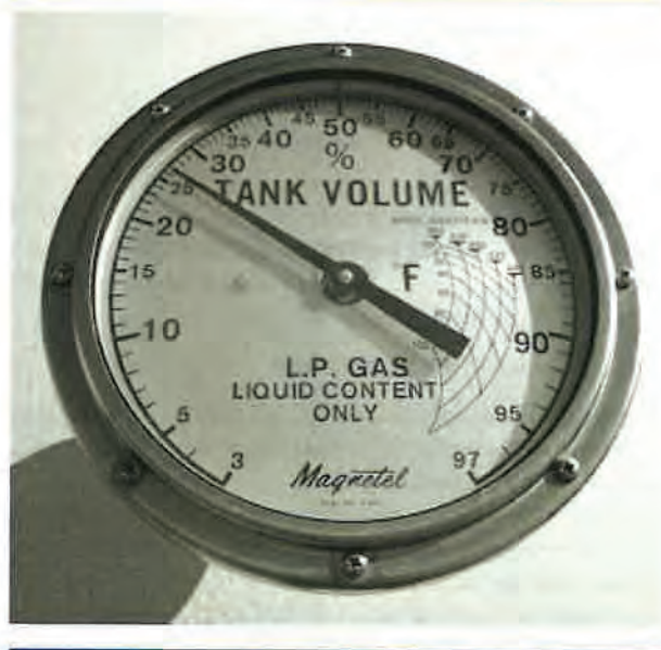
EXHIBIT 5.43 Variable Liquid Level Gauge. (Courtesy of Eastern Propane Corp.)
