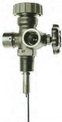
EXHIBIT 5.41 Multiple Valve for 100 lb to 200 lb (45 kg to 91 kg) Cylinder with Fixed Maximum Liquid Level Gauge (Dip Tube) and Separate Inlet and Outlet Connections. (Courtesy of Sherwood, Harsco Gas & Fluid Control Group)
