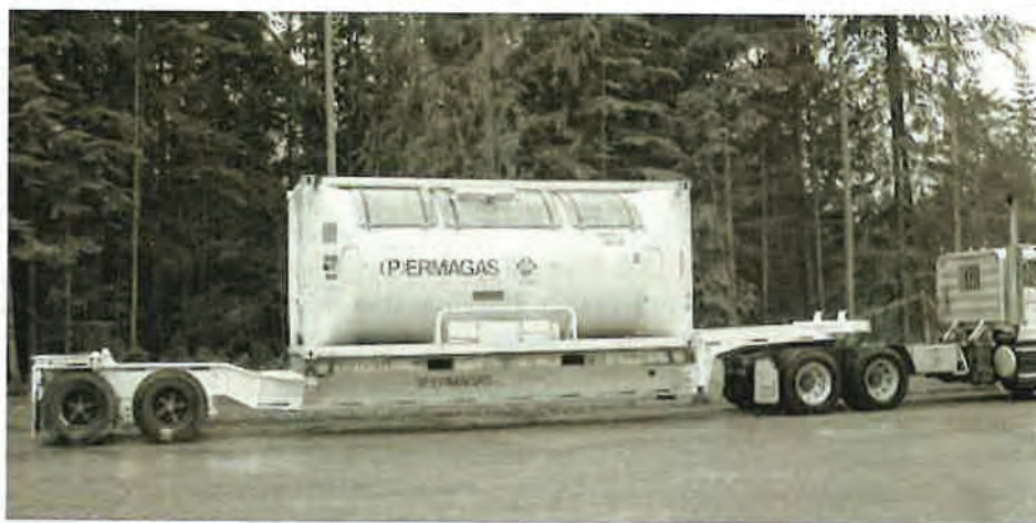
EXHIBIT 5.6 Intermodal Container. (Courtesy of Permugas)
