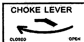
Figure 7 - Choke in the close position
