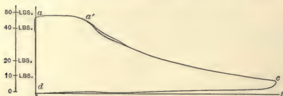
FIG. 1-32. — Diagram from Brayton Working Cylinder.
