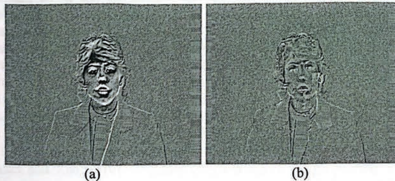
Figure 3.5 (a) Interframe and (b) motion compensated interframe pictures
