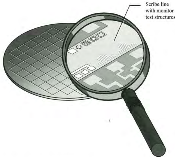
FIGURE 19.3 Scribe Line Monitor Test Structure
