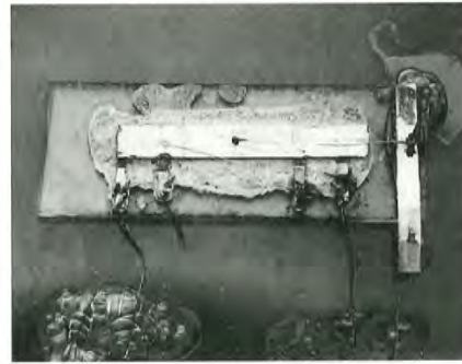
Jack Kilby's First Integrated Circuit (Photo courtesy of Texas Instruments, Inc.)
