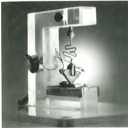
The First Transistor from Bell Labs (Photo courtesy of Lucent Technologies, Bell Labs Innovations)
