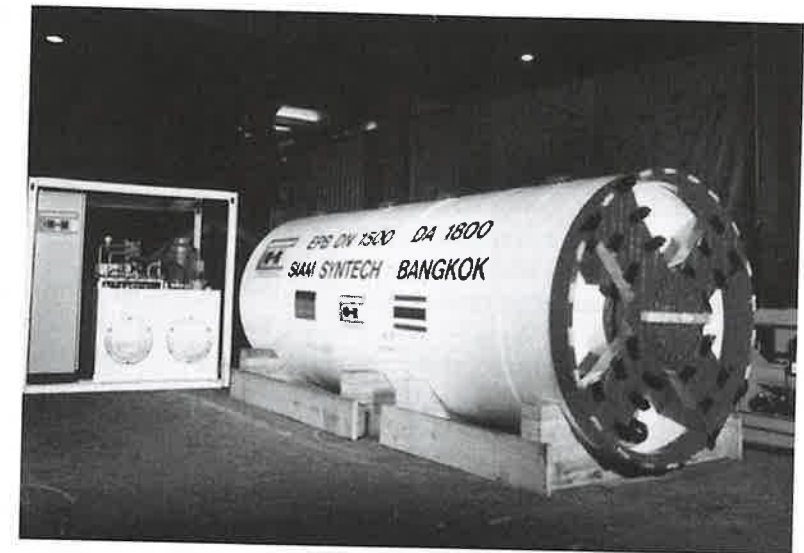
FIGURE 12.7 A horizontal earth-boring machine used for installing pipes. (Courtesy of Herrenknecht Company and Ruhr-University of Bochum, Bochum, Germany.)
