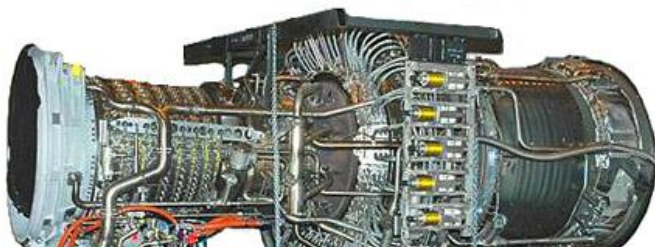
LM2500 STIG Aeroderivative Gas Turbine Package (30 MW)
