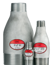
Swage Nipples Sizes: 1/8" – 8" Thickness: STD, XH and XXH End Connections: TBE, THD x BEV MSS-SP-95
