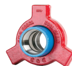
Figure 1002 10,000 PSI NSCWP Sizes 1" – 5", Threaded or Butt Weld 6", Butt Weld 5" Threaded @ 5,000 PSI NSCWP 5" and 6" Butt Weld @ 7,500 PSI NSCWP
