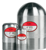
Bull Plugs Sizes: 1/4" – 8" Thickness: STD, XH, XXH Threaded Zinc Plated Available with Taps MSS-SP-95
