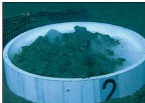
Figure 6.10 Liquid CO 2 released at 3600 metres initially forms a liquid CO 2 pool on the sea floor in a small deep ocean experiment (upper picture). In time, released liquid CO 2 reacts with sea water to form a solid CO 2 hydrate in a similar pool (lower picture).
