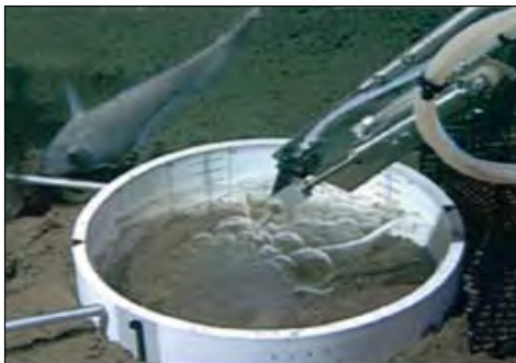
Figure 6.10 Liquid CO 2 released at 3600 metres initially forms a liquid CO 2 pool on the sea floor in a small deep ocean experiment (upper picture). In time, released liquid CO 2 reacts with sea water to form a solid CO 2 hydrate in a similar pool (lower picture).
