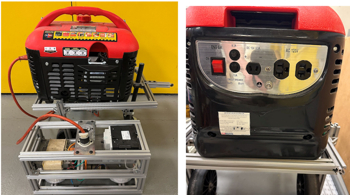
Portable Generator for Robotic Mobile Boom Crane.
