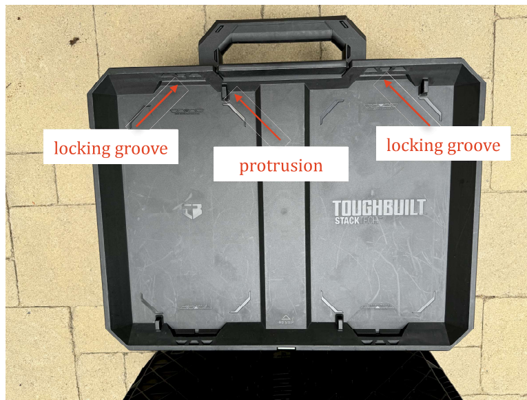
(a). The lower storage box showing the protrusion that trips the detent to cause the cleats to engage the locking grooves.
