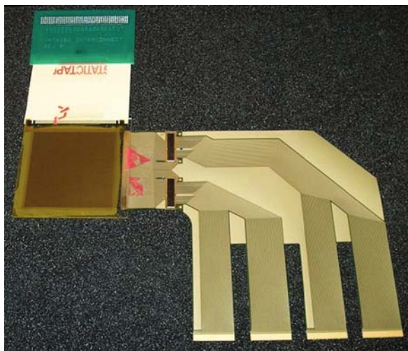
Fig. 4.10 160 \times 160 (\times 3) pixel display connected to the COF column drivers and flex cable connected to a row driver board
