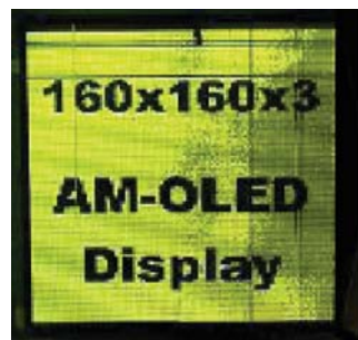
Fig. 4.12 Photograph of a text image being displayed on a 160(\times 3) \times 160 pixel AMOLED fabricated using a flexible PEN plastic backplane built with low-temperature a-Si TFTs
