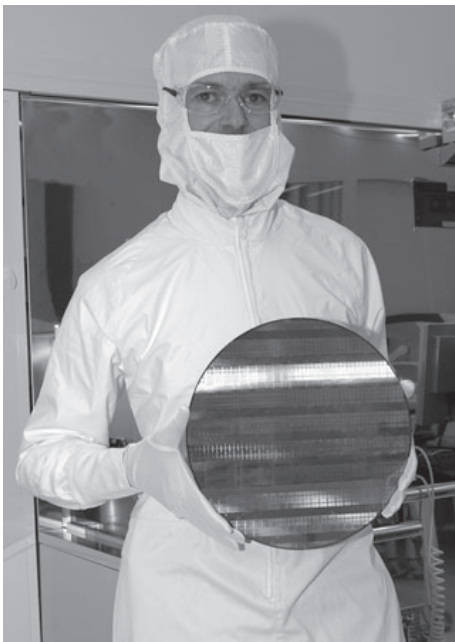
FIGURE 1.71 Engineer holding processed 12-inch wafer (Photograph courtesy of the Intel Corporation.)
