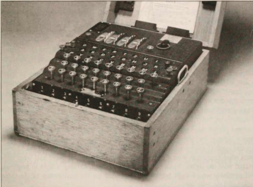
Figure 18-1. An Enigma Machine
