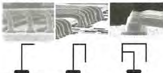
FIGURE 9A-4 Loop height reduction using the capillary. (Courtesy of K&S.)
