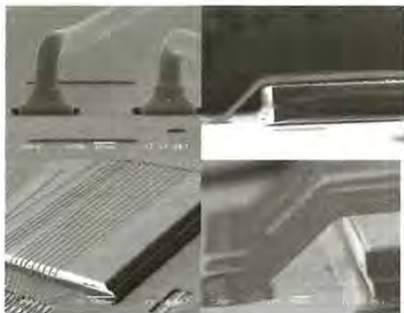
FIGURE 9A-2 Examples of long low loops. (Courtesy of Oerlikon.)
