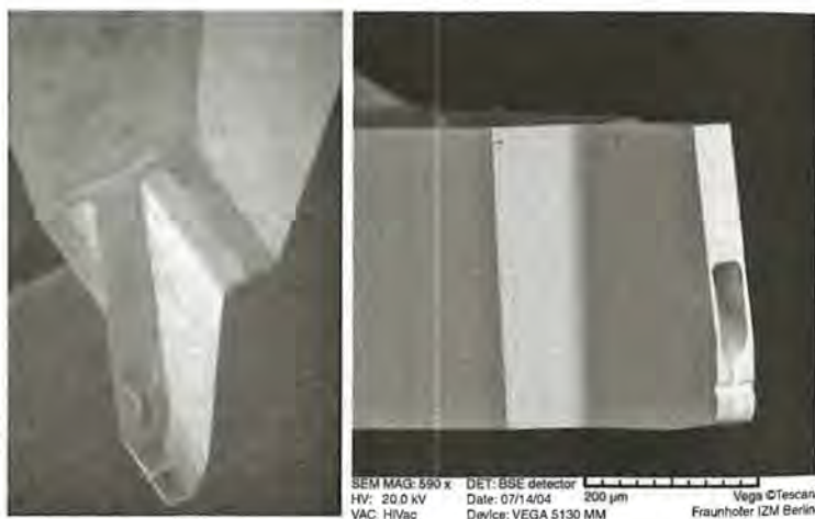
FIGURE 9-9 Fine-pitch wedge bonding tools. The left is an older design. (Courtesy of Microminiature Tech.) On the right is a recent design that is stronger (less fragile). This tool has a cross-groove in its foot, and is intended for fine-pitch wedge bonding with gold wire. (Courtesy of Fraunhofer IZM.)
