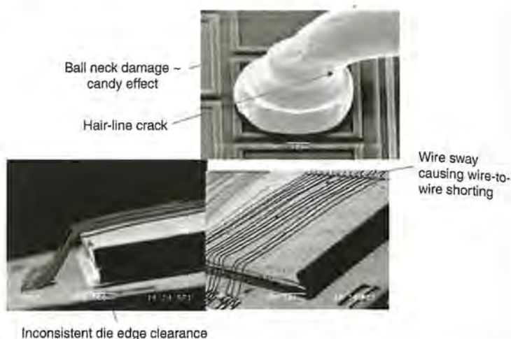
FIGURE 9A-6 Wire bond loop defects. (Courtesy of Oerlikon.)
