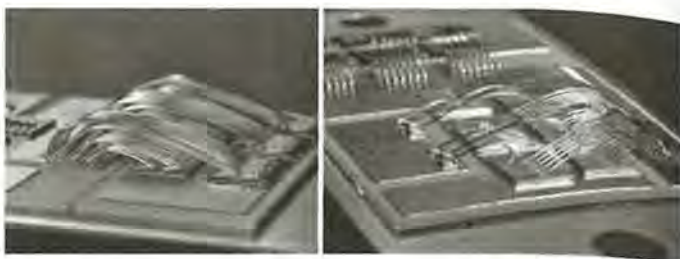
FIGURE 9A-9 Heavy wire wedge and ribbon bonding. (Courtesy of Orthodyne.)
