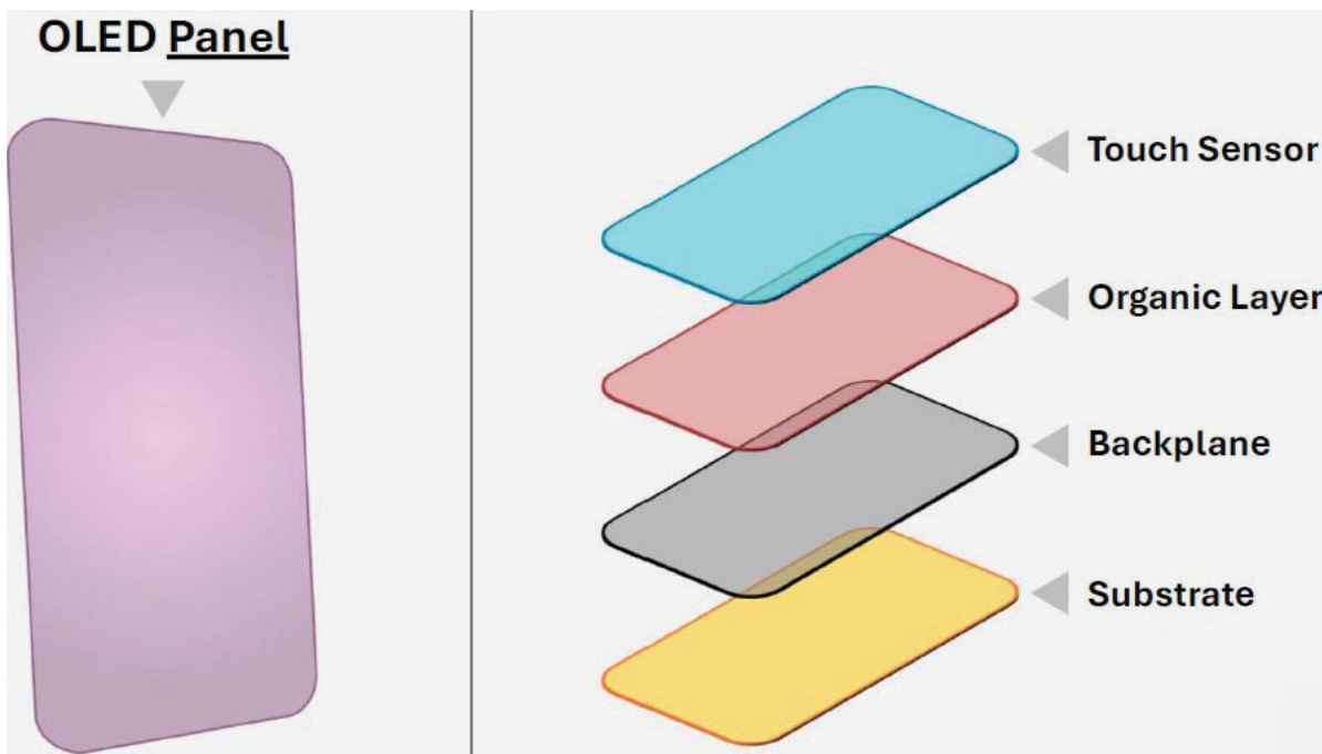
Figure 4: Layers of an OLED Panel
