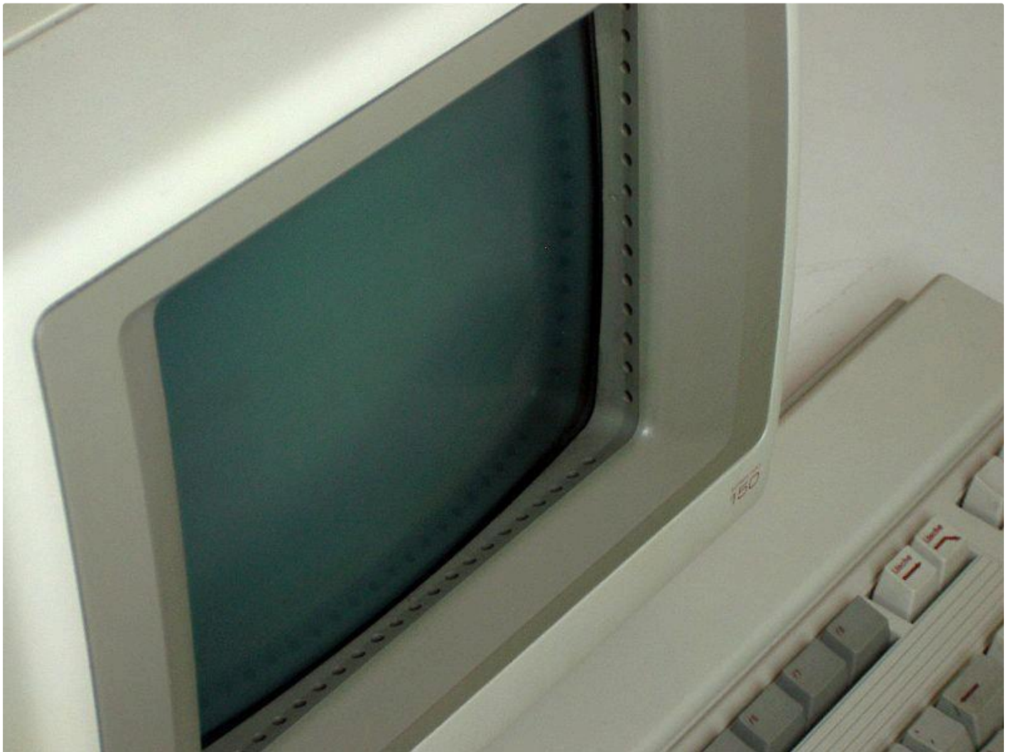
The HP-150 featured MS-DOS and a 9-inch touchscreen Sony CRT. Credit: Wikimedia Commons
