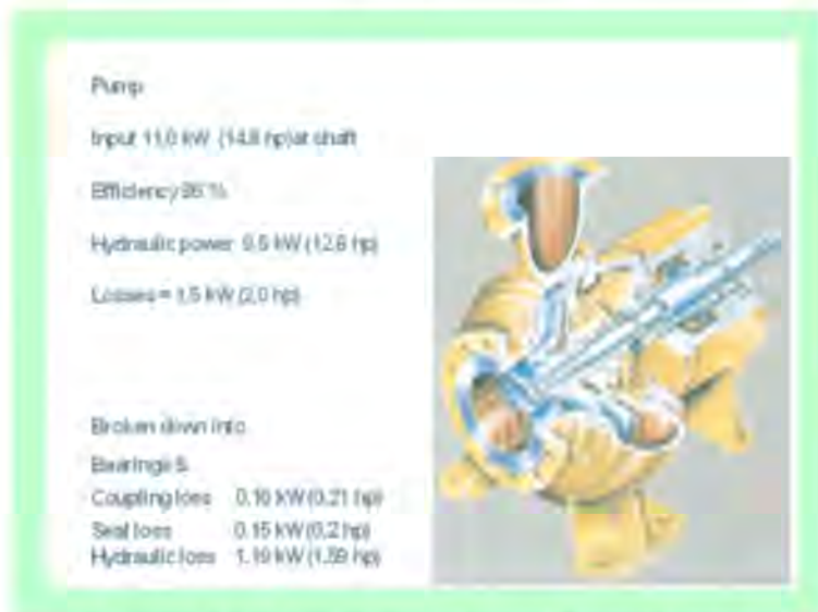
Figure A6.2: Typical rotodynamic pump losses
