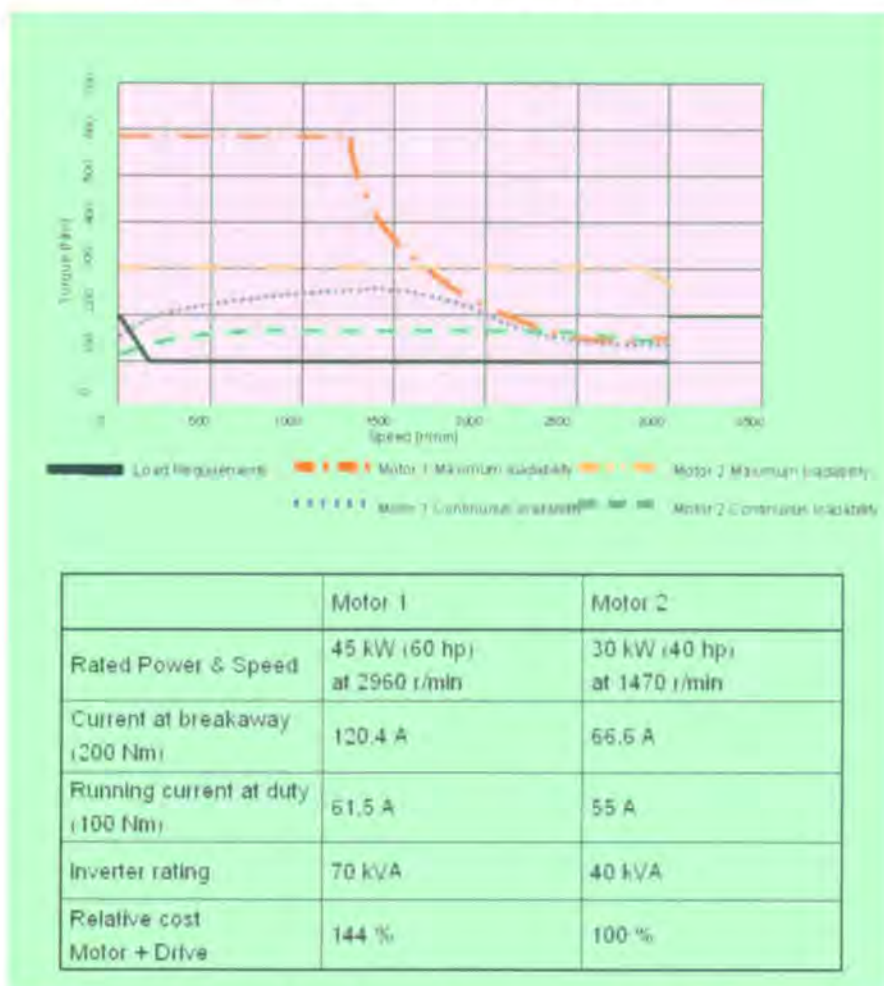
Figure 11.4: Motor load capacity curves
