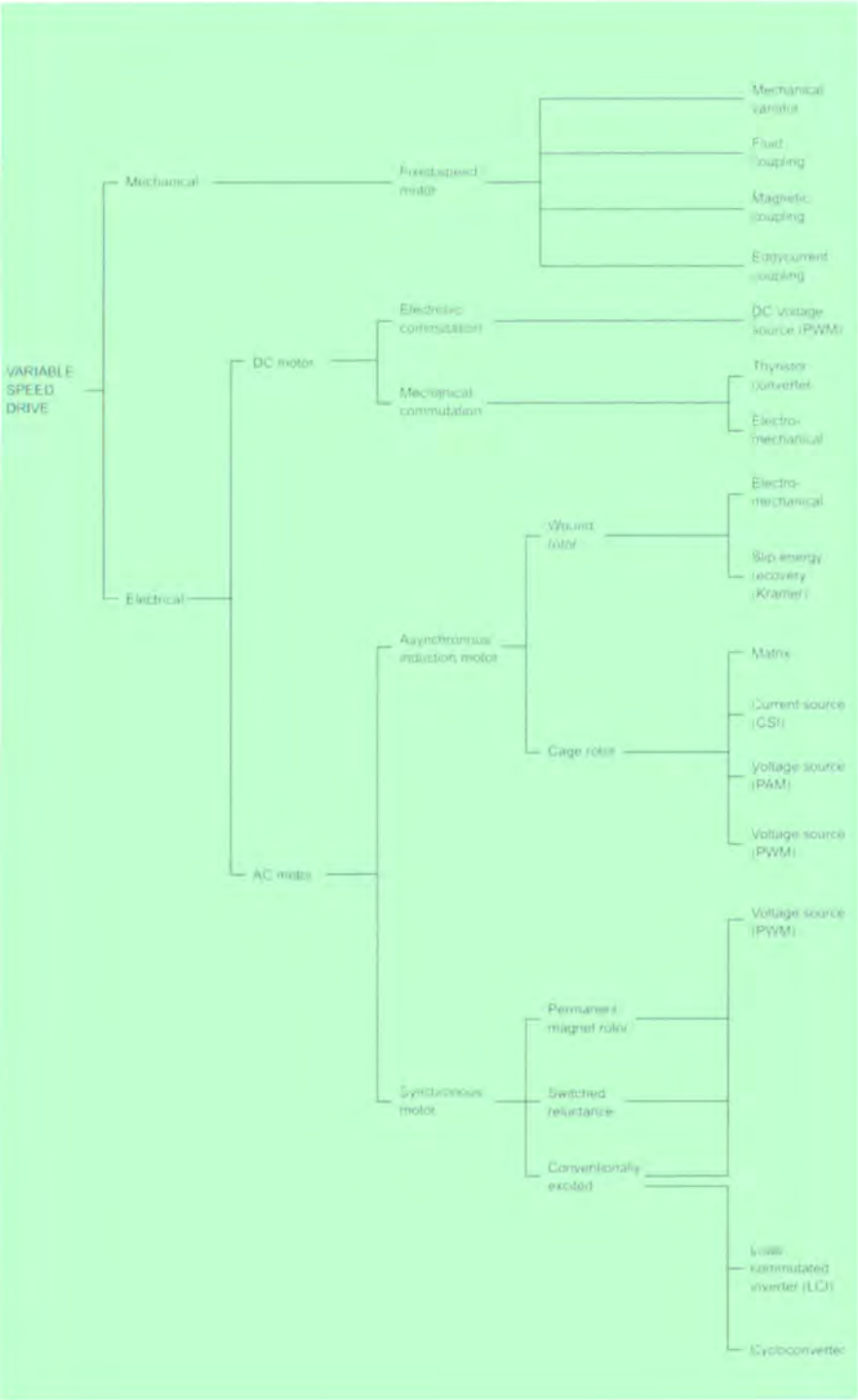
Figure 7.1: Types of variable speed drive (VSD)
