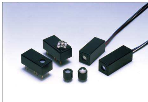
Figure 4.26. Compact PMTs and modules containing the PMTs. The diameter of the PMT is 16 mm. The width of the PMT modules is 25 mm. Courtesy of William Cieslik, Hamamatsu Photonics Systems.
