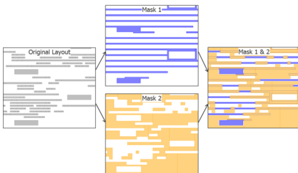
Figure 3: SADP masks compared to the original drawn layout.
