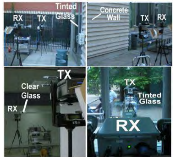
FIGURE 5. Images of the 28 GHz reflection measurement for outdoor tinted glass at ORH (top left), outdoor concrete wall at ORH (top right), penetration loss measurement for indoor clear non-tinted glass at MTC (bottom left) and tinted glass at ORH (bottom right) [28].
