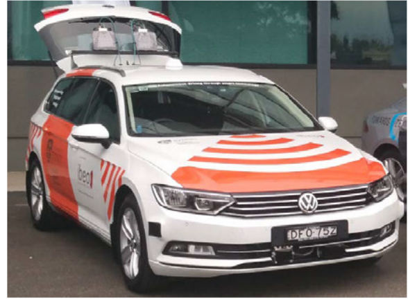
Fig. 1. Vehicle fitted with GPS that allows for filtered GPS position, heading and speed to be recorded for experiments. It is also fitted with a 360 degree coverage lidar based perception system from Ibeo Automotive Systems GmbH [3], allowing for real-time detection and tracking of neighbouring vehicles. The vehicle is fitted with a DSRC radio allowing for communication between vehicles.
