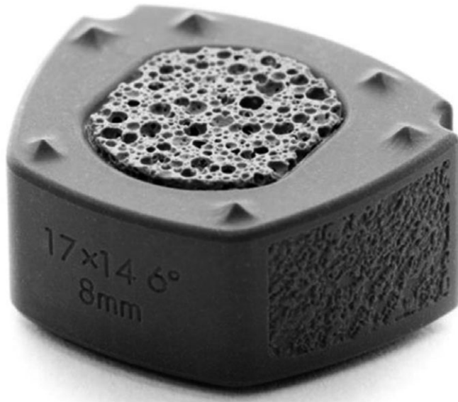
Fig. 7 A composite silicon nitride cervical implant (photograph courtesy of Amedica Corporation, Salt Lake City, UT, USA) 17 .
