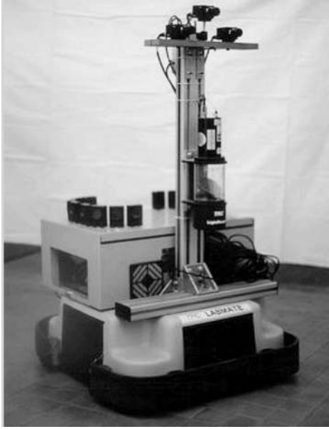
Figure 12. The vehicle is square with differential traction and equipped with a laser 3D TRC.
