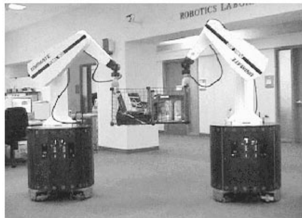
Fig. 1. The Stanford robotics platforms: two holonomic platforms, each is equipped with a PUMA 560 arm, various sensors, two computer systems, a multi-axis controller, and sufficient battery power to allow for autonomous operation.
