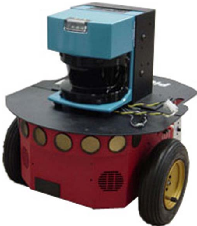
Figure 4 Pioneer 3 with SICK laser
