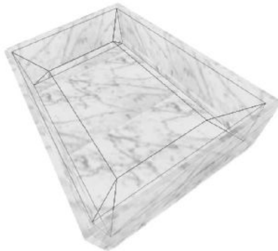
Figure 5.15 The solid lines represent the GVG for a rectangular enclosure whose ceiling has been removed to expose the interior. Imagine a sphere rolling around touching the removed ceiling, floor, and side wall; the center of this sphere traces a GVG edge.
