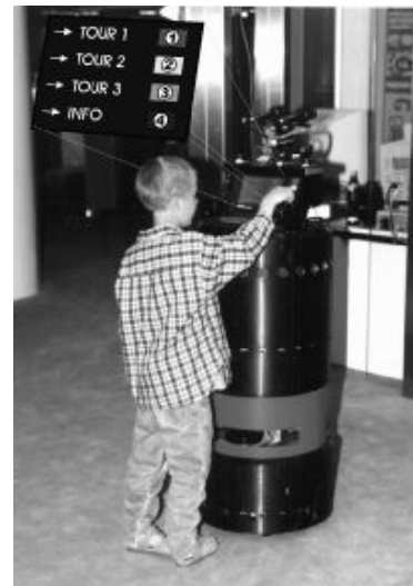
Figure 1.3 RHINO, the interactive mobile tour-guide robot.
