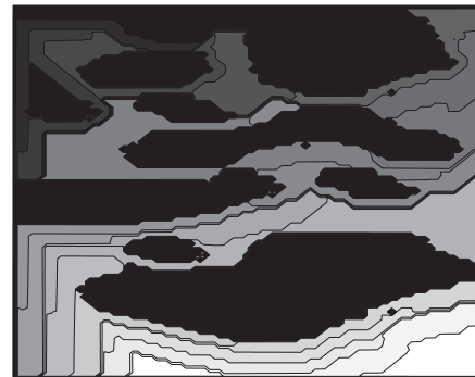
Figure H.9 A plot of linklength values from the start (upper left corner) node where colored pixels correspond to link lengths of paths defined by the depth-first search. The lighter the pixel the greater the linklengths in the graph; black pixels correspond to obstacles.
