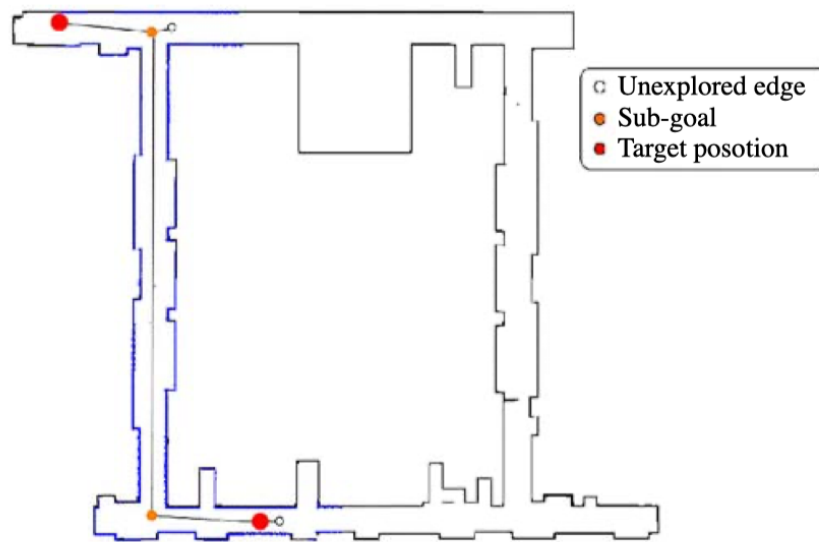
Figure 19 The topological map constructed by the proposed path planner
