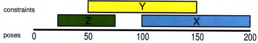
Figure 5-1: Three overlapping constraints. A disturbance in constraint X will be propagated through Y to Z, even though X and Z do not overlap. At each step, the effect of the disturbance is attenuated.
