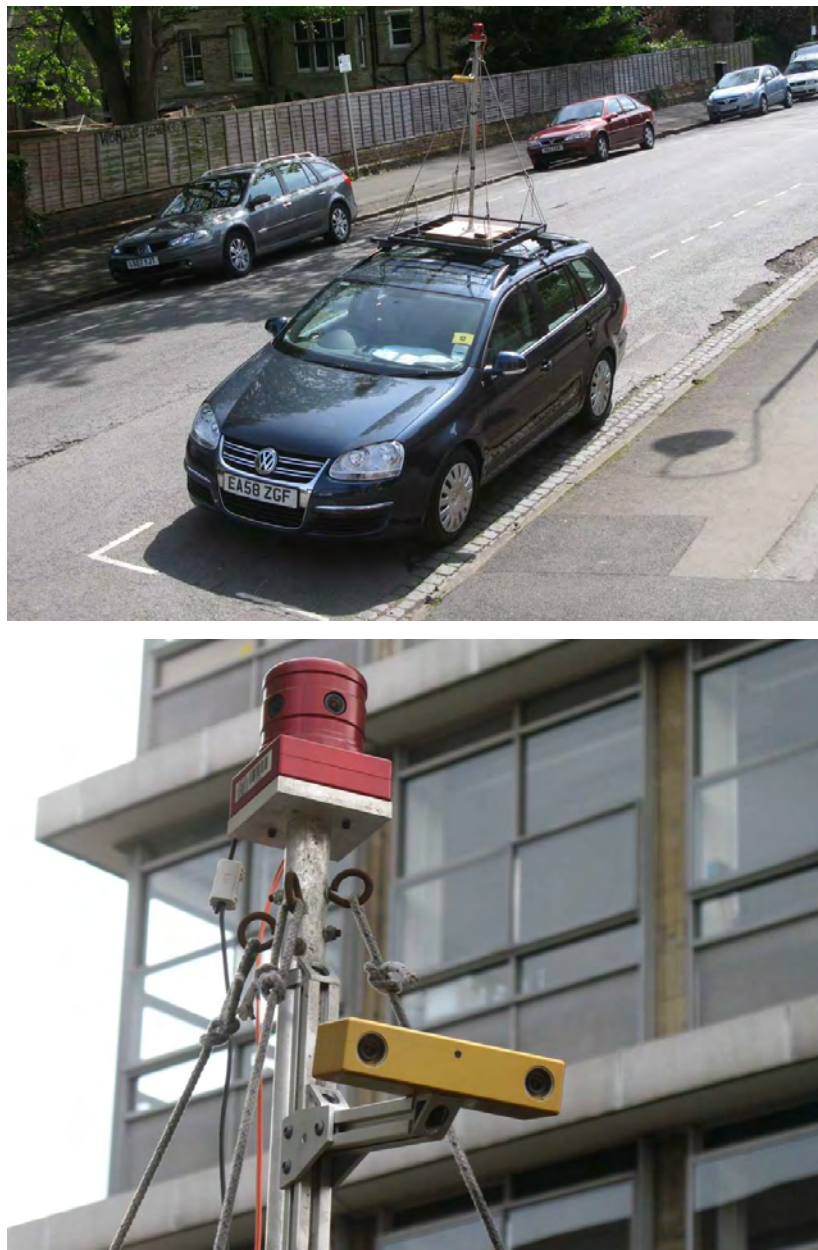
Figure A.2: Vehicle and sensor rig used to capture the 70 km and 1,000 km data sets used in Chapter 5.
