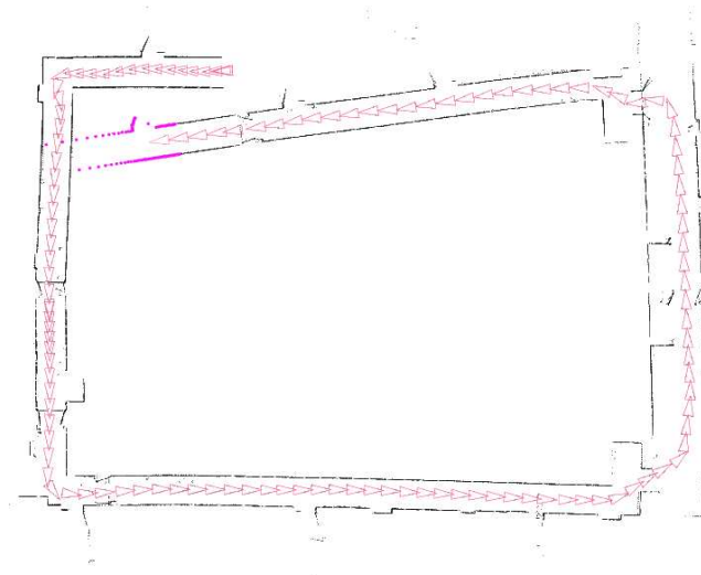
Figure 2.2: A example of loop closure detection failure in an indoor environment. Triangles show vehicle poses. As the robot travels along the corridor, linearization and perception errors accumulate. When the robot returns to the starting point, its true location lies outside the three-sigma bound on vehicle uncertainty (not shown). The nearest neighbour data association technique fails, and the robot's map becomes corrupted. (Figure courtesy of Oxford Mobile Robotics Group)
