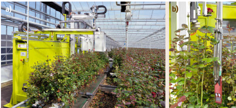
Fig. 56.20a,b A rose harvesting robot. (a) The robot with the rose crop on a mobile growing system. (b) The end-effector with stereo vision system and a scissors-type cutting device (courtesy Jentjens Machinetechniek BV, Veghel, The Netherlands)
