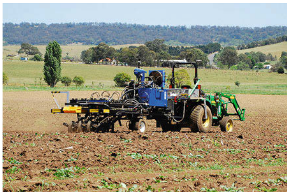
Fig. 56.7 Precision seeding system for broad acre farming
