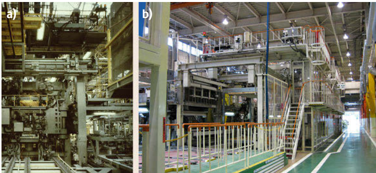
Fig. 57.9 (a) Sequencing station; (b) robotic assembly system for vertical brickwork layering; (c,d) final brickwork panel product
