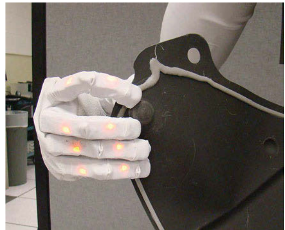
Fig. 41.14 Robot exploring a 2-D deformable object (after [41.59])
