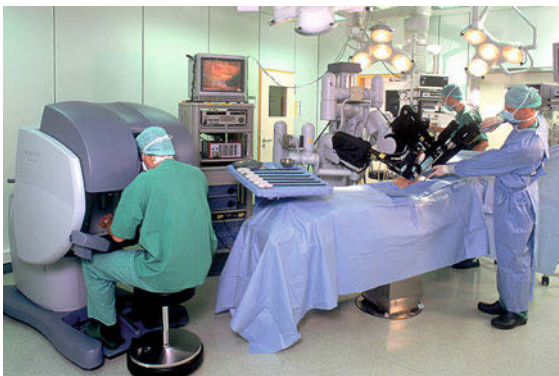
Fig. 43.7 Intuitive Surgical Inc. makes the da Vinci telerobotic system, which is used in minimally invasive surgery (courtesy 2008 Intuitive Surgical, Inc.)
