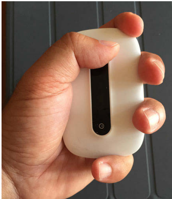
Fig. 38.6 The palm and fingers combine to create a very secure form closure grasp of a router
