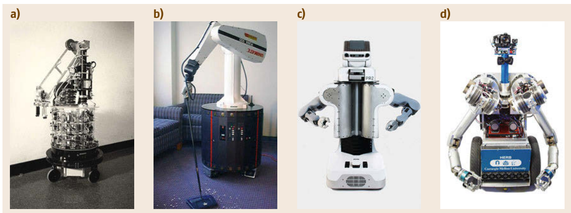
Fig.40.1a–d Some exemplary mobile manipulation platforms developed throughout the decades (a) Herbert (MIT, 1985), (b) Stanford assistant mobile manipulator (1995), (c) PR2 (Willow Garage, 2009), (d) Herb (CMU, 2013)
