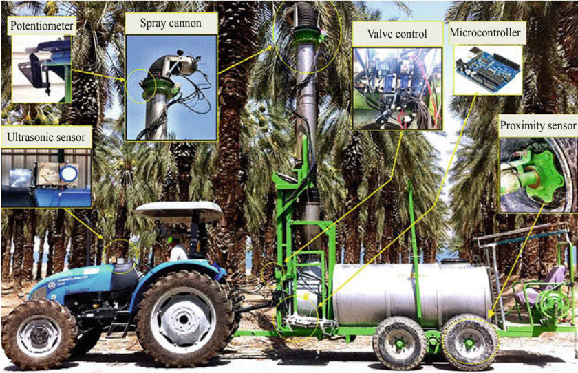
Fig. 56.14 Date tree tracking system adapted to a commercial sprayer. The system aims the sprayer nozzle toward the trees more efficiently and safely than a human operator
